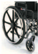
24" x 1" solid tyred molded Mag. rear wheels; 8" x 1" solid tyred casters
