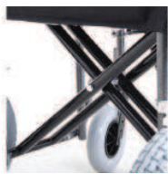
Reinforced double cross-braces
