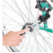
24" x 1-3/8" PU tyres with quick release axle
