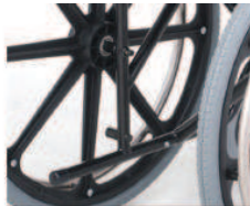
Universal design with two axle bushings
